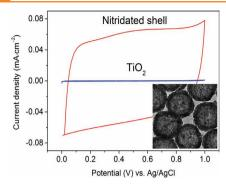
Hollow shells of TiO2 are nitridated by annealing in NH3, assembled into a monolayer film on water surface, and stacked layer-by-layer into electrodes for electrochemical energy storage. This approach facilitates supercapacitor cell design by simplifying the electrode structure and avoiding the use of any organic binder or carbon-based conducting materials. The increased electrical conductivity due to the formation of TiN greatly enhances the electrochemical performance.
