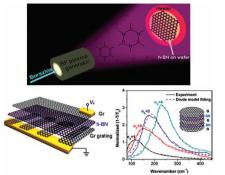
An array of graphene/h-BN vertically stacked micrometer-sized disks is fabricated by lithography and transfer techniques, and infrared spectroscopy is used to observe the modes of tunable graphene plasmonic absorption as a function of the repeating (G/h-BN)<sub>n</sub> units in the vertical stack.
