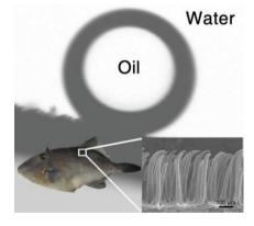
Unique anisotropic underwater oleophobicity of the skin of filefish Navodon septentrionalis is revealed, which results from its oriented hook-like spines. Inspired by this, an anisotropic underwater oleophobic surface is fabricated on an oxygen plasma-treated PDMS layer. Anisotropic microfeatures on the surfaces and hydrophilicity are proposed as two main factors in achieving anisotropic underwater oleophobicity.
