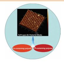
Rapid single-step fabrication of large-area nanodot arrays of L10-FePt nanoparticles (NPs) are achieved by employing a metallopolymer blend of individual Fe- and Pt-containing homopolymers as the precursor through nanoimprint lithography. Imaging of the nanodot pattern indicates that the patterned NPs exhibit a decent magnetic response, which suggests potential to be utilized directly in the fabrication of bit-patterned media for the next generation of magnetic recording technology.
